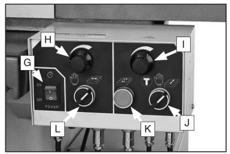
Figure 3. Power feed controls.
